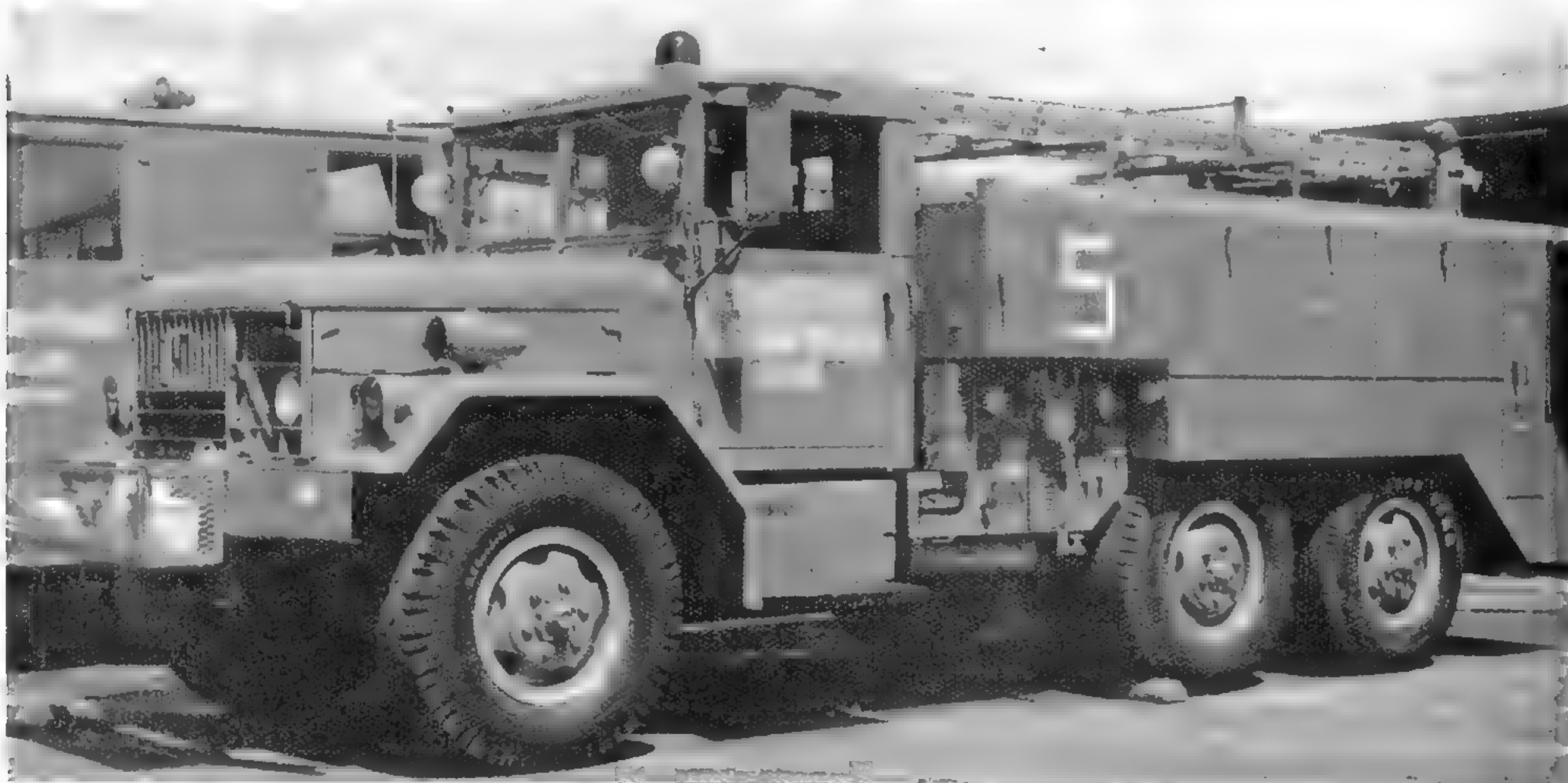
The 530B retained the single 11.00-20 tires of the 530A, but featured a new enclosed bed and a midship-mounted pump. (Photo courtesy of Richard Adelman collection)
